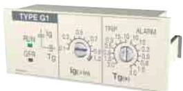
The ground fault protection (GFR) of several hundred amperes is possible. This function can be selected for trip and alarm (no trip). Power supply is necessary for this function, even if there is no power supply, it can function at  $0.2 \times I_n$  or higher.
