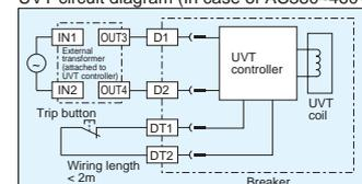
Note 1) In case of 380-460V AC, the external transformer is attached.
