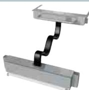
With the breaker taken out of its cradle, this device enable the breaker to be electrically opened and closed, and the operating sequence to be checked. 3m length one is equipped as standard shipment.
