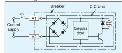
Diode rectifier is not used for control source 24-48V DC.
