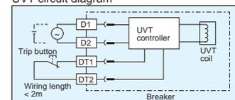
UVT circuit diagram (In case of AC380-460V)
