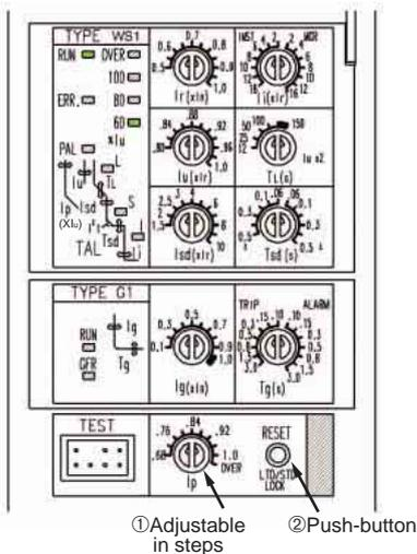
4 When the characteristics is set up, use a device like a field tester, etc to make sure that the required characteristic has been set.
