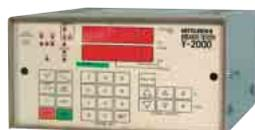
The field test device (Y-2000) can be checked the Electronic Trip Relay function at test position and disconnected position.
