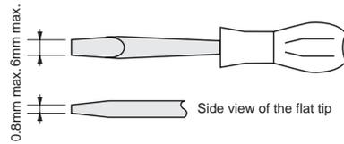
2 Insert the flat tipped screwdriver into the opening of the ETR cover. Then, lightly turn the screwdriver to the upside as shown in the left figure, and the relay cover will open.
