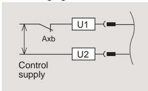
A OFF charging method is also available. The closing spring is charged automatically when the breaker is opened. This is available only by externally connecting in series b contact (AXB) of the auxiliary switch to the motor charging circuit. In case of DC power supply, please use high capacity auxiliary switch (HAX).
