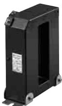
The Neutral CT is used for ground fault protection when the 3 pole breaker is used on a 3 phase 4 wires system and for over current protection on N phase. Please use this CT in combination with ground fault protection (GFR). As for outline dimensions, refer to page 48.
